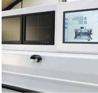
Up to 2000 jobs can easily be registered in the operator panel of the FlexMount. Data can be retrieved and uploaded as spread sheets.
