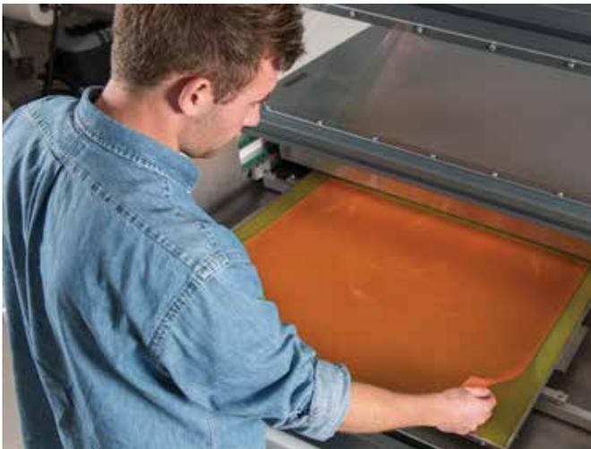
Ergonomically optimized with low input height and simple plate handling during daily operation.
