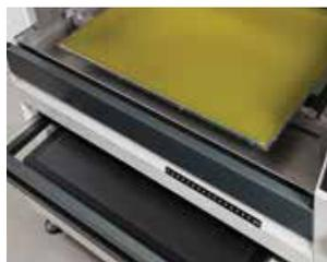
▲ Cooled exposure bed for consistent exposure results.
